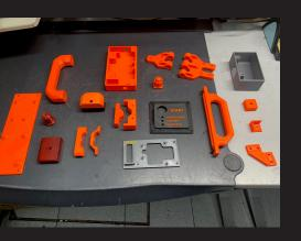
Additive manufacturing enables us to produce each component to the exact specification and purpose, and enables the use of bespoke components where normally just the tooling costs would be impossible to bear on a project of this nature. Specific polymers can be chosen for each purpose, such as highly resistant PETG for external parts, UV resistant ASA for items close to the light source and high detail, environmentally friendly PLA for cosmetic parts.
